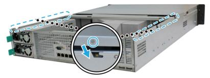
**b** Put back and fasten the screw you removed in step 2.
